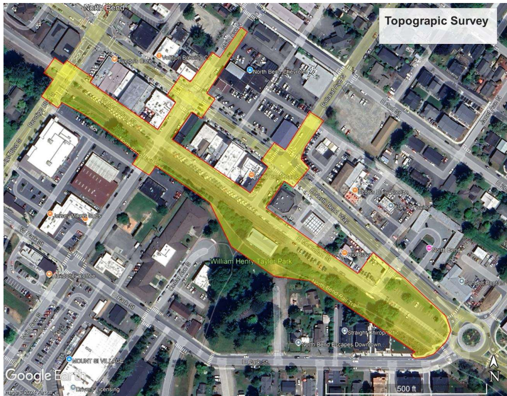
Figure 1 – Project Topographic Survey Limits & Right of Way Limits. The east end of the project area (Ballarat Ave N to E. Park Street) was surveyed by Survey and Mapping (SAM) and will be used as a reference check but will not be merged into the new base map. The horizontal datum used will be NAD 1983/91 and the vertical datum used will be NAVD 88. The Consultant will provide a detailed survey basemap in AutoCAD, version 2024.
