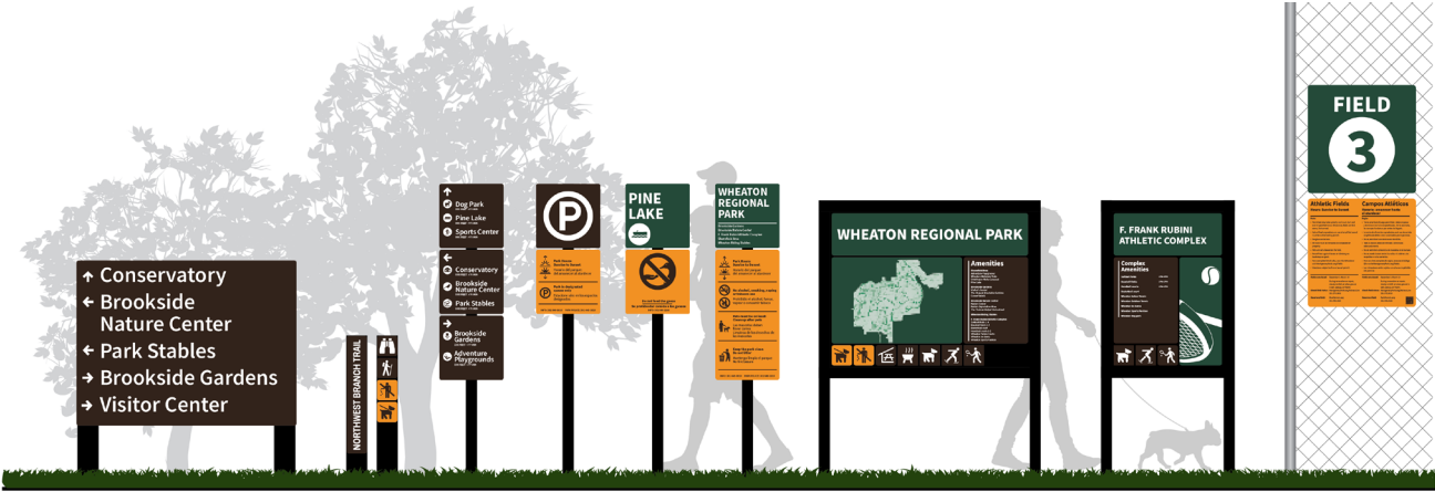
Above: Examples of sign panels on a 6" module with 1/2" spacing, allowing for easy combination and development of new sign types Below: Examples of mounted sign panels in typical arrangements
